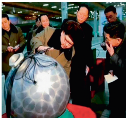
Figure 3 Examining a DPRK spherical probable fission device with only 12 cables entering the metal case around the high explosives
