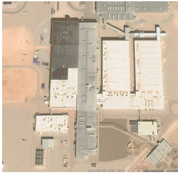
Figure 1. The addition of similar plant modules to increase plant capacity is clear in the evolution of the Urenco centrifuge separation plant at Eunice, New Mexico, USA
