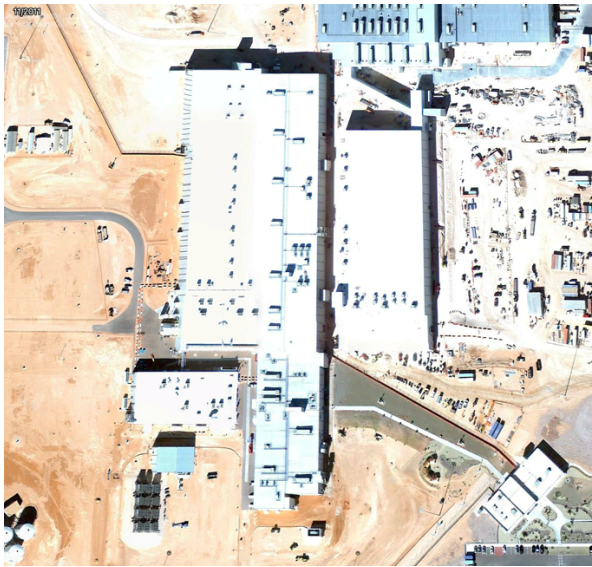
Figure 1. The addition of similar plant modules to increase plant capacity is clear in the evolution of the Urenco centrifuge separation plant at Eunice, New Mexico, USA
